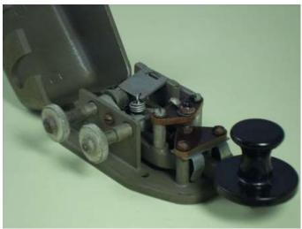
The second model (dating from the 2nd World War and after?) has a molded metal base, without any parts attached with screws on the base.
